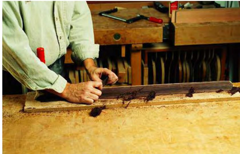
7-3 Scraping with grain to remove plane marks
