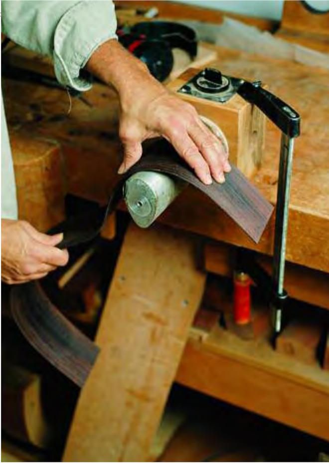
**7-5** Keep the wood moving on bending iron
