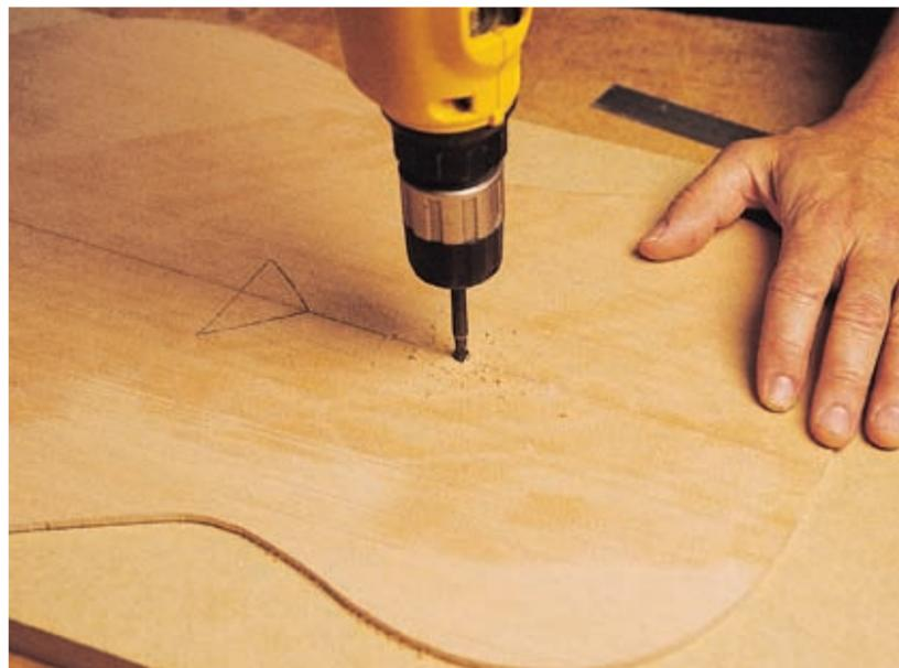
9-16 Drilling hole for dowel
