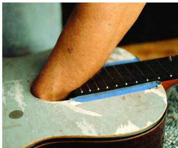
**14-32** Taping caul to the underside of the top
