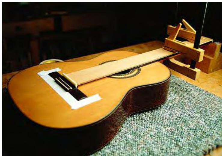
**14-28** Positioning bridge with bridge stick clamped to fingerboard
