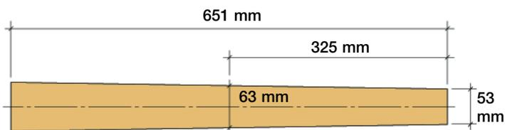
Note: Tapered as fingerboard, continue taper to saddle.
